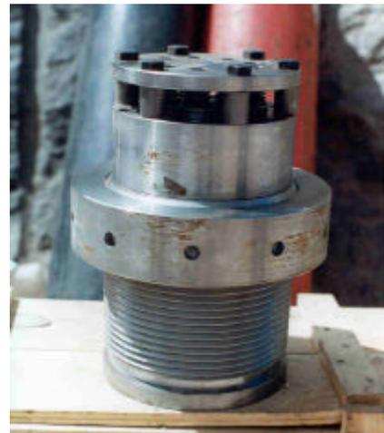
Figura 26. Anclaje regulable
