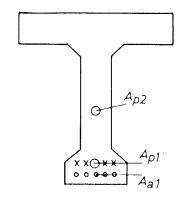
.ARMADURA NO PRETENSADA:  $A_{01}$  ADHERENTE ARMADURA PRETENSADA:  $A_{p1}$  ADHERENTE ARMADURA PRETENSADA:  $A_{p2}$  NO ADHERENTE
