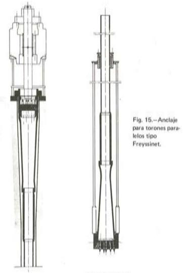
ANCLAJE SUPERIOR E INFERIOR Y GATO DE TENSION
