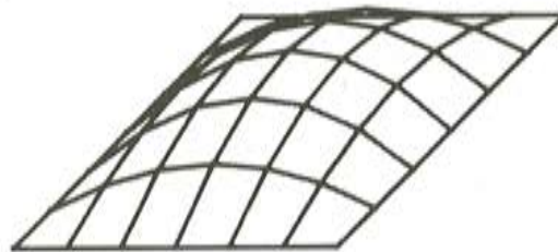
Velaria paraboloidal A = B = 2, C = 1, m = -\frac{2C}{B} = -1
