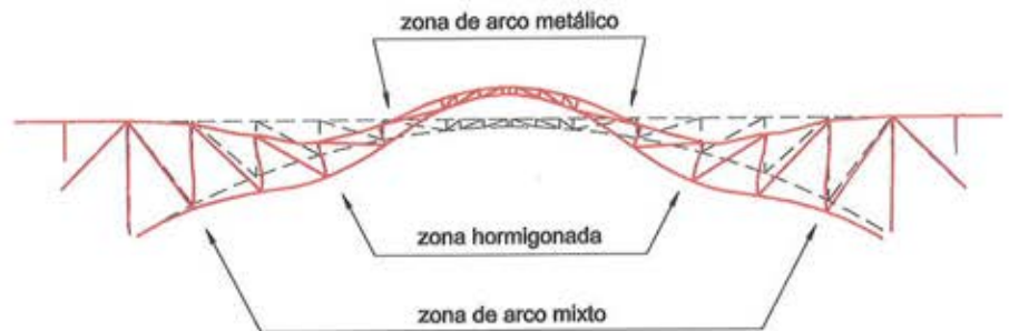
Figura 16. Hormigonado 2.º tercio sin regulación de diagonales. Figure 16. Concreting the second third, without cross beam regulation.
