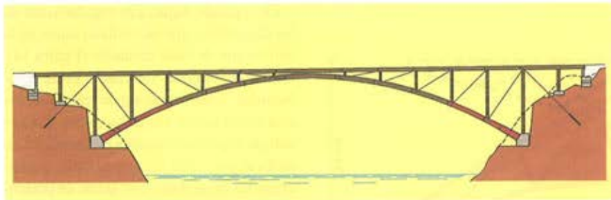
Figura 12. Hormigonado del 1 er tercio del arco. Figure 12. Concreting the first third of the arch.
