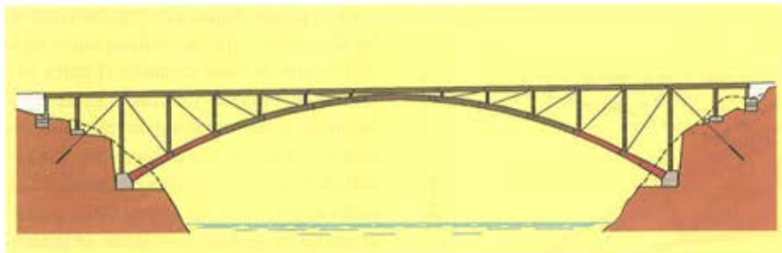
Figura 12. Hormigonado del 1 er tercio del arco. Figure 12. Concreting the first third of the arch.
