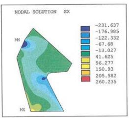
Figura 16. Estado tensional del capitel. Figure 16. Pier head tensional state.
