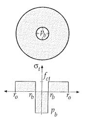
$$\sigma_{t}(r) = p_{b} \frac{r_{b}^{2}}{r_{o}^{2} - r_{b}^{2}} \left( 1 + \frac{r_{o}^{2}}{r^{2}} \right)$$
