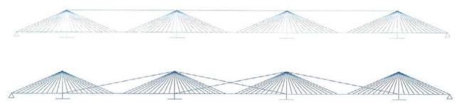
Figura 33. Puentes atirantados continuos con tirantes adicionales de rigidización de pilonos. Figure 33. Continuous cable stayed bridges with additional stays for pylons stiffening.
