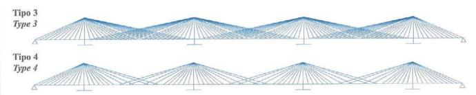
Cont. Figura 44. Modelos de puente atirantado continuo con tirantes adicionales cruzados. Cont. Figure 44. everal continuous cable stayed bridges with additional crossed stays.
