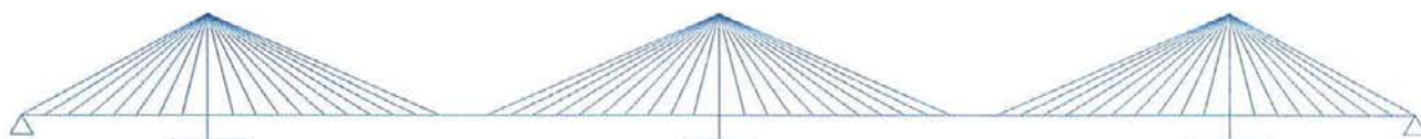
Figura 27. Puente atirantado continuo de 4 vanos con vanos laterales descompensados y pilonos de igual altura. Figure 27. Four span continuous cable stayed bridge with lateral unbalanced spans and pylons of the same height.
