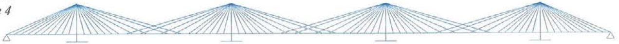
Cont. Figura 44. Modelos de puente atirantado continuo con tirantes adicionales cruzados. Cont. Figure 44. everal continuous cable stayed bridges with additional crossed stays.
