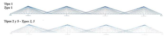
Figura 44. Modelos de puente atirantado continuo con tirantes adicionales cruzados. Figure 44. Several continuous cable stayed bridges with additional crossed stays.
