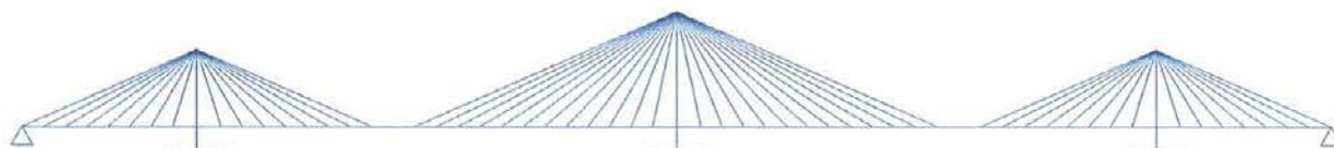
Figura 28. Puente atirantado continuo de 4 vanos con vanos laterales descompensados y pilono central de mayor altura que los laterales. Figure 28. Four span continuous cable stayed bridge with lateral unbalanced spans and a central pylon higher than the others.
