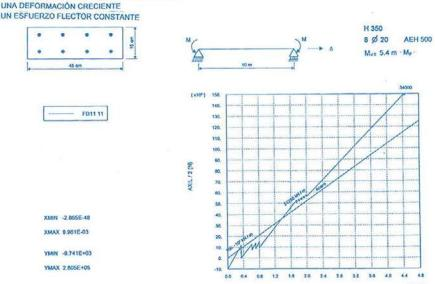
Figura 19. Diagrama axil deformarado en varios tirantes. Figure 19. Diagram axia force I— deformation of several ties.
