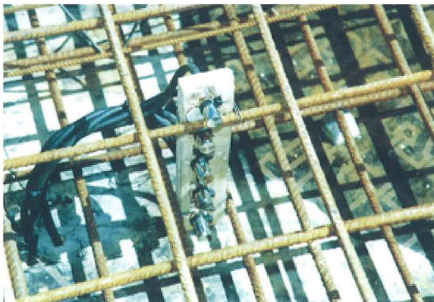
Figura 26. Transductor de desplazamiento. Figure 26. Measuring of deformations.
