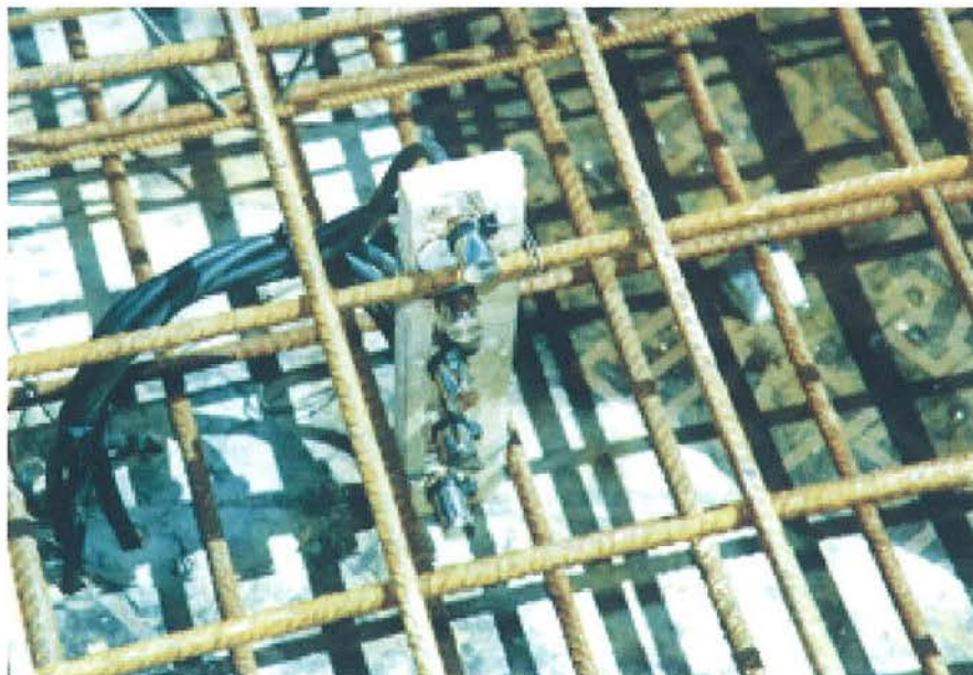
Figura 26. Transductor de desplazamiento. Figure 26. Measuring of deformations.
