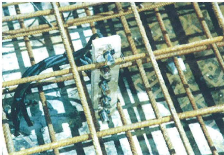
Figura 26. Transductor de desplazamiento. Figure 26. Measuring of deformations.
