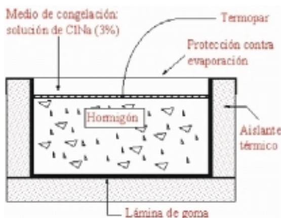
Fig. 24: Ensayo hielo-deshielo (salt scaling). Detalle de la probeta y resultados. Fig. 24: Freezing and thawing (salt-scaling) test —detail of test specimen and results.
