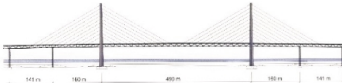
Fig. 6: Alzado del puente principal atirantado del Puente de Öresund. Fig. 6: Side view of the main cable-stayed bridge of the Öresund Link.
