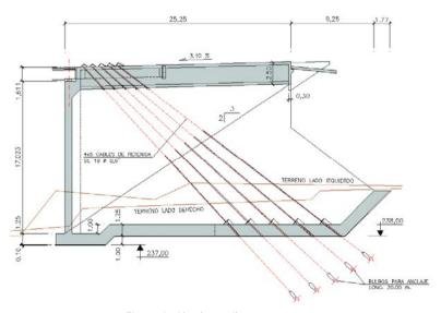
Figura 8. Alzado estribo norte. Figure 8. North abutment drawing.
