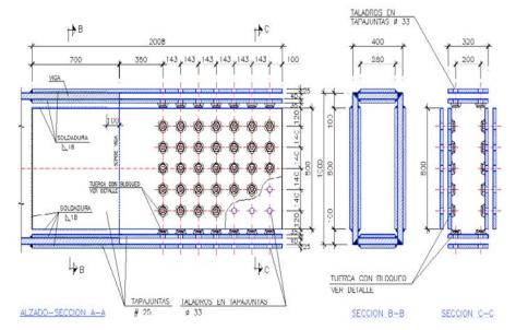
Figura 7. Uniones vigas principales. Figure 7. Main beam unions.
