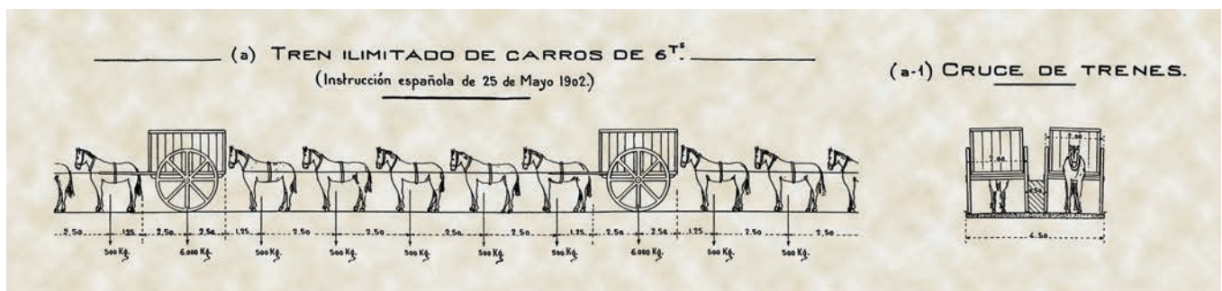
Figura 8. Tren de cargas original. Figure 8. Original truck loads.
