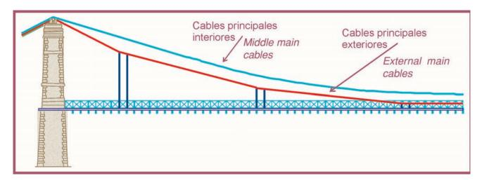
Figure 12. Destesado total de cables a retirar: principales interiores, tirantes y de retenida. Figure 12. Total de-tensioning of cables to be removed: middle main cables, stays and guylines.
