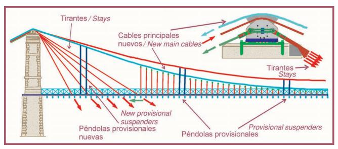
Figura 22. Montaje y tesado de tirantes, cables de retenida y cable horizontal. Figure 22. Mounting and tensioning stays, guylines and horizontal cable.
