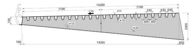
Figure 15. Alzado de ménsula lateral. Figure 15. Front view of lateral cantilever.
