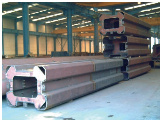
Figura 38. Tramos en taller preparados para el transporte Figure 38. Stretches in shop prepared for shipping
