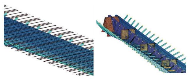
Figuras 22 y 23. Modelo de elementos finitos. Cálculo transversal Figures 22 and 23. FEM model for the calculations of transverse effects
