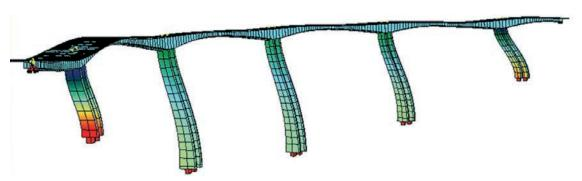
Figura 10. Modelo de cálculo de subestructura Figure 10. Structural model for the calculation of the piers
