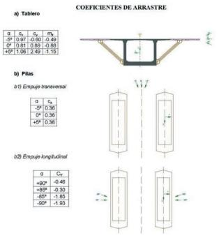
Figure 9. Wlid pressure coefficients of the deck and of the piers
