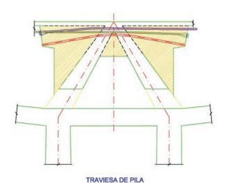
Figura 24. Macizado zona superior de la traviesa de pila Figure 24. Concrete extension of the connection of the deck to the pier
