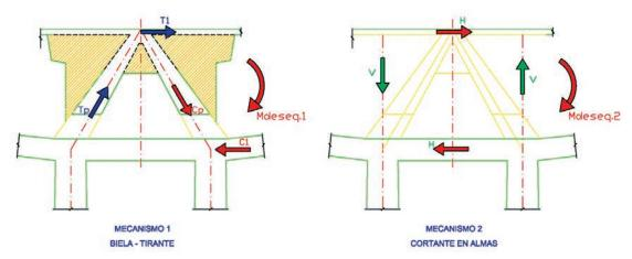
Figure 25. Doble mecanismo resistente de la traviesa de pila Figure 25. Two different structural system of the connection of the deck to the piers
