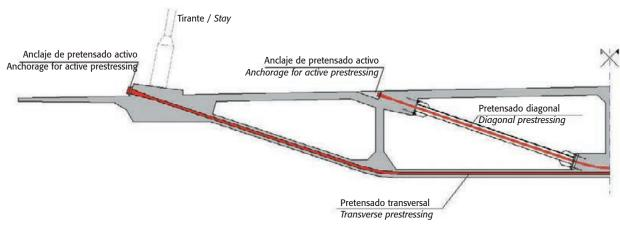
PRETENSADO TRANSVERSAL ALZADO / TRANSVERSE PRESTRESSING ELEVATION VIEW
