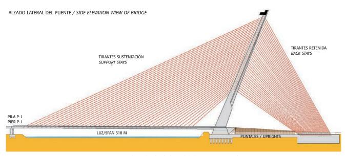
Figura 2. Plano de alzado lateral del puente atirantado Figure 2. Side elevation view of the cable-stayed bridge
