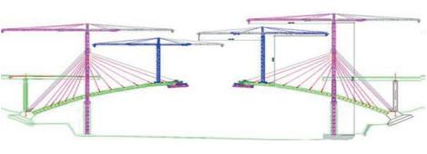
Figura 18. Atirantamiento provisional Figure 18. Temporary staying
