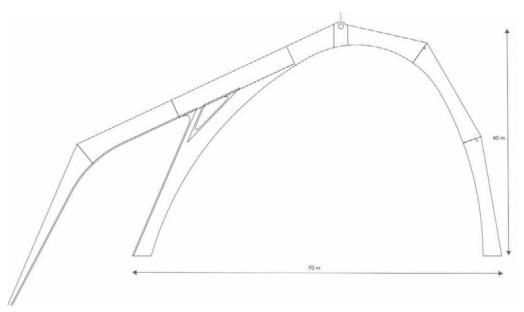
Figura 17. Alzado de la costilla fija CF-0 Figure 17. Lateral view of the fixed rib CF-0
