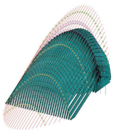
Figure 37. Perspective of the general model with the roof closed
