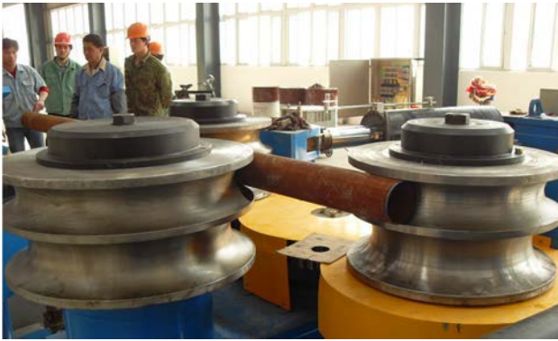
Figura 31. Curvado de tubos Figure 31. Tube curving
