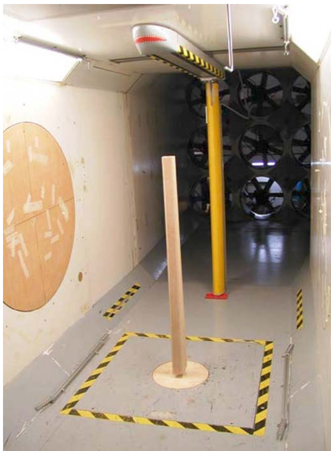
Figure 12. Cross-sectional wind test on pier 4.
