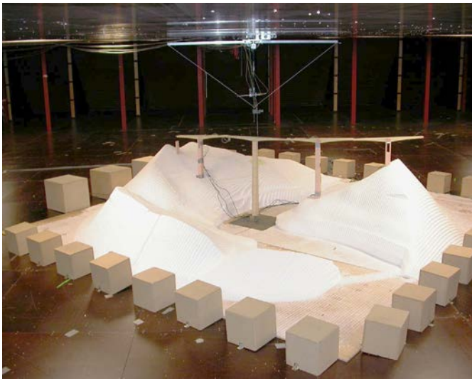
Figure 15. Scale model of bridge under construction for wind tunnel test.
