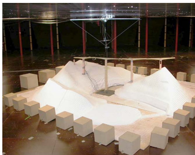
Figure 15. Scale model of bridge under construction for wind tunnel test.
