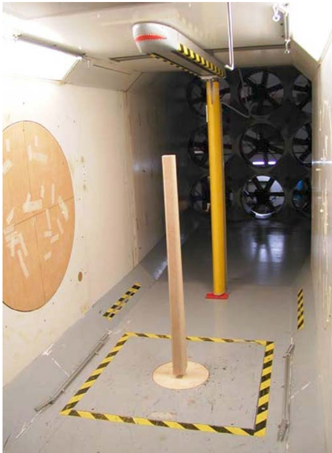
Figure 12. Cross-sectional wind test on pier 4.
