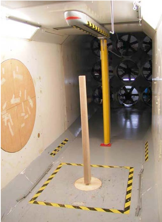
Figure 12. Cross-sectional wind test on pier 4.
