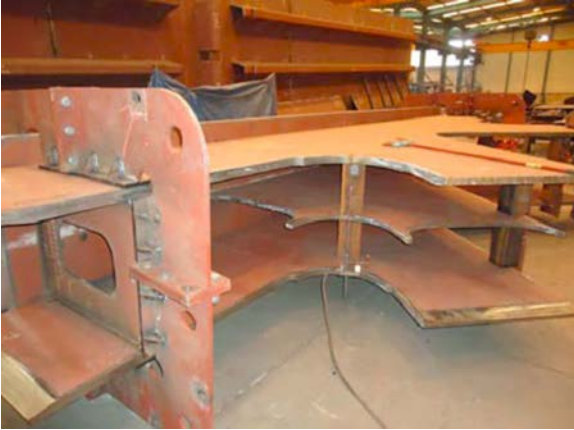
Figure 15. Manufacture of a recumbent node.
