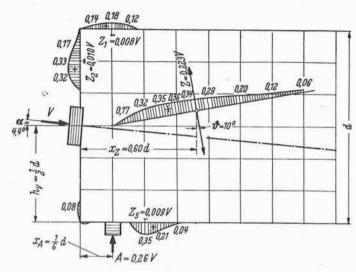
FIG. 9.  $h_v = \frac{1}{2} d$ ,  $x_A = \frac{1}{6} d$ , A = 0.26 V (MODELO 2, ENSAYO 7)
