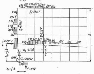
$h_v = \frac{1}{3} d$ ,  $x_A = \frac{1}{6} d$ , A = 0.1 V (MODELO 1, ENSAYO 2)
