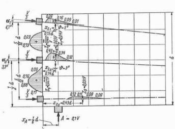
FIG. 19.  $h_{V~(m)} = \frac{1}{2} d, \quad x_A = \frac{1}{6} d, \quad A = 0.1~V$  (MODELO 5, ENSAYO 17)
