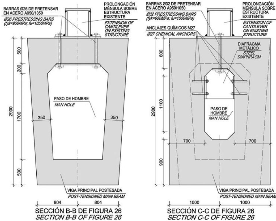
Figure 27. Anchored length of cantilevered by-pass (cross-sections).
