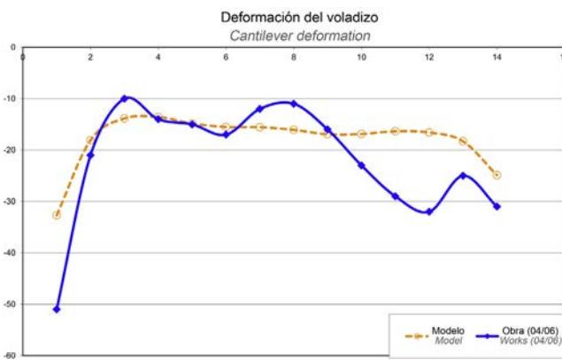
Figure 59. Comparison of cantilever movements after roof de-bracing.
