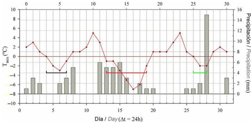
Figure 14. Procedure used to determine maximum monthly snowfall [12].
