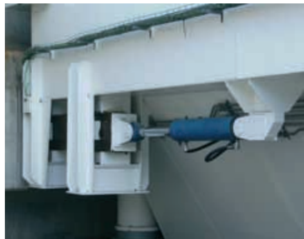
Figura 20. Enclavamiento dorsal. Figure 20. Rear interlocking
