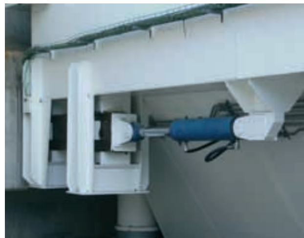
Figura 20. Enclavamiento dorsal. Figure 20. Rear interlocking
