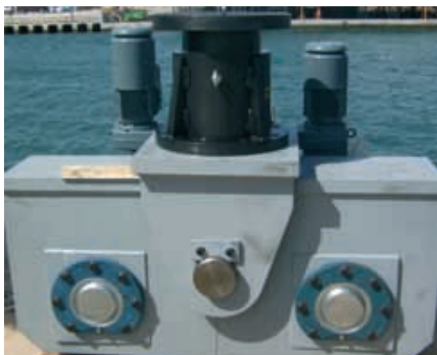
Figuras 12 y 13. Carretones de apoyo dorsal. Figures 12 and 13. Bearing traction wheels at rear of bridge.
