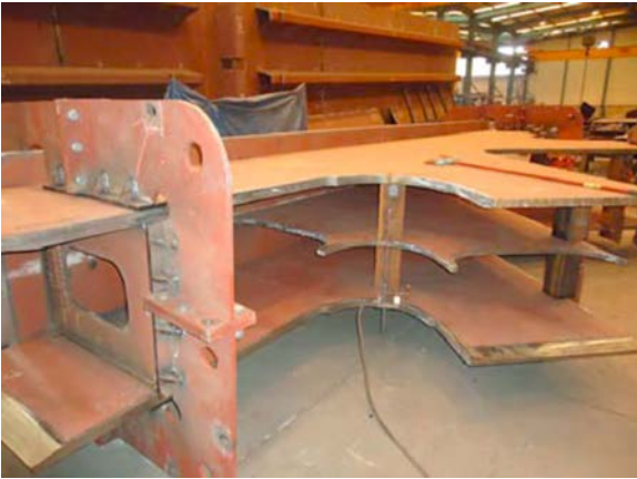
Figure 15. Manufacture of a recumbent node.
