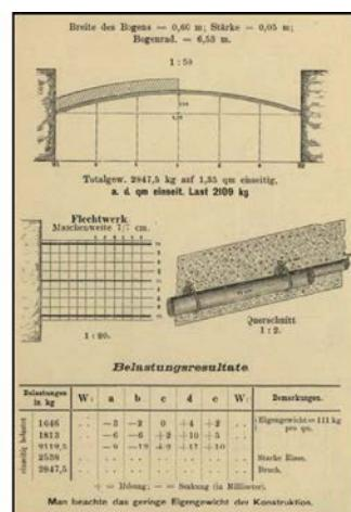
Figure 4. Ribera's Reservoir in Gijón in 1902, and the Monier system for the vaults.
