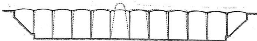
Figure 9. Deformation of the roof faced with thermal increase in accordance with the publication by Fritz von Emperger.
