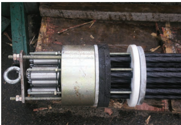
Figura 27. Nuevo anclaje superior con manguitos Figure 27. New top unions equipped with extrusion sleeves
