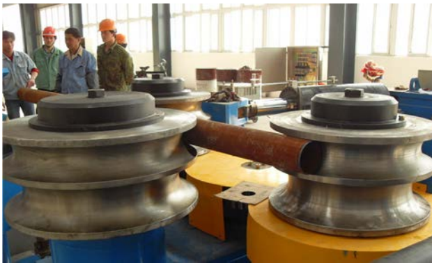
Figura 31. Curvado de tubos Figure 31. Tube curving
