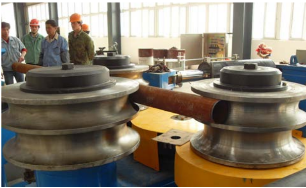
Figura 31. Curvado de tubos Figure 31. Tube curving
