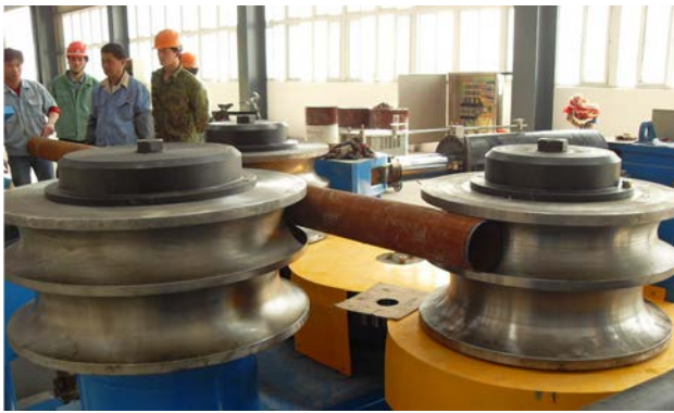
Figura 31. Curvado de tubos Figure 31. Tube curving
