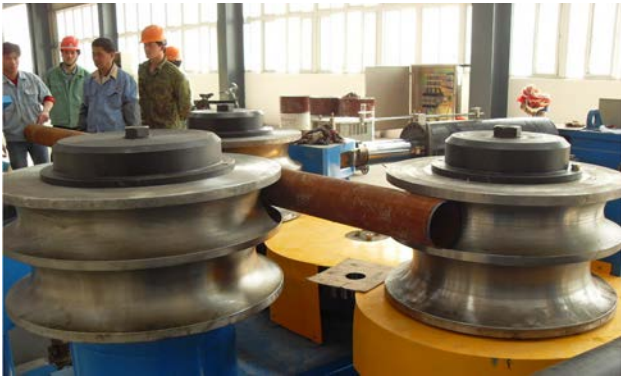
Figura 31. Curvado de tubos Figure 31. Tube curving
