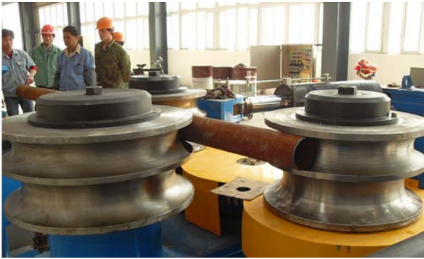
Figura 31. Curvado de tubos Figure 31. Tube curving
