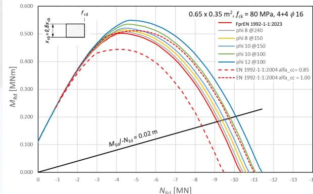
Note consistency between capacity based on parabola-rectangle and based on stress block
