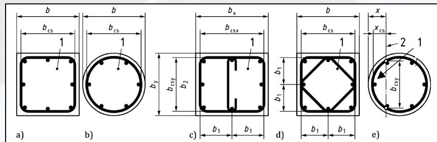
*N.B.: Effect of confinement on the strain limits in concrete may be considered according to Formulae (8.16) and (8.17) but exclude concrete areas outside confining reinforcement*
