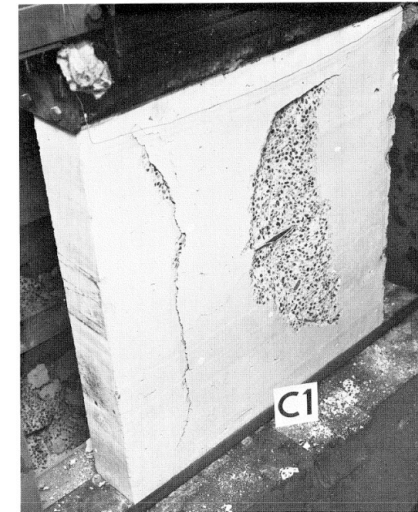
Fig. 1. Slab-type lightweight concrete specimen after a fire test.
