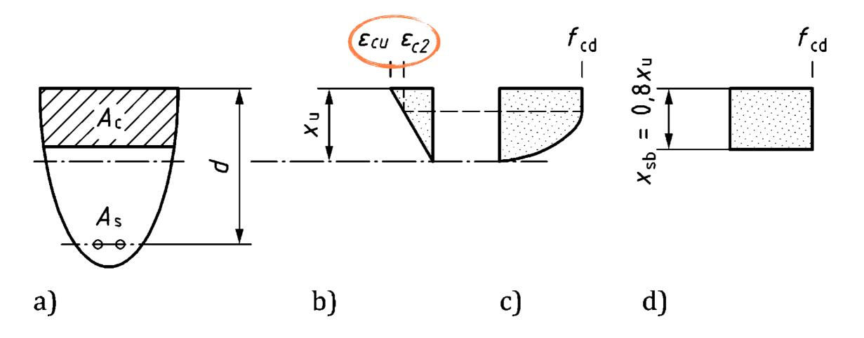
These parameters are 0.0020 and 0.0035 respectively, for concrete without fibres.
