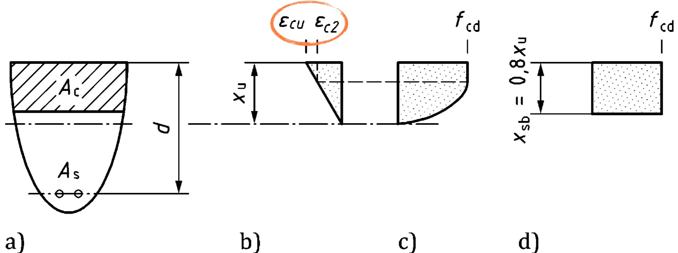
These parameters are 0.0020 and 0.0035, respectively, for concrete without fibres.
