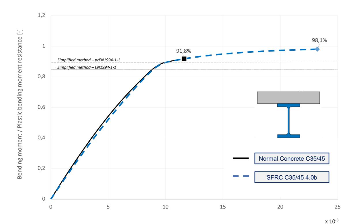
Curvature of the cross-section [1/m]
