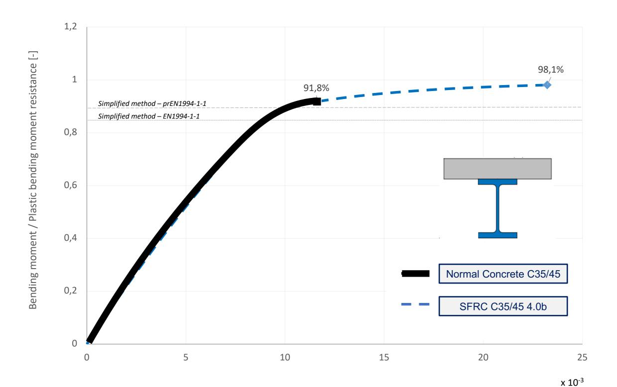
Curvature of the cross-section [1/m]
