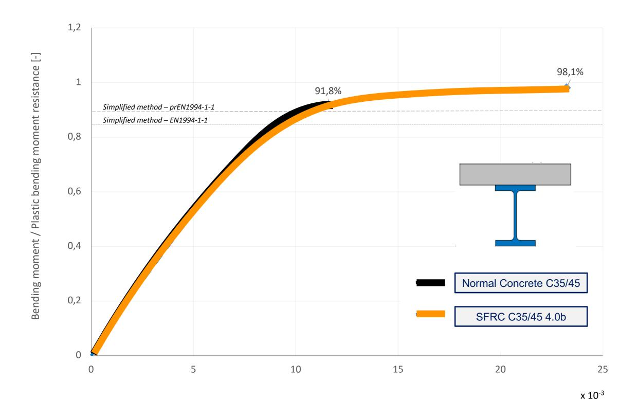
Curvature of the cross-section [1/m]
