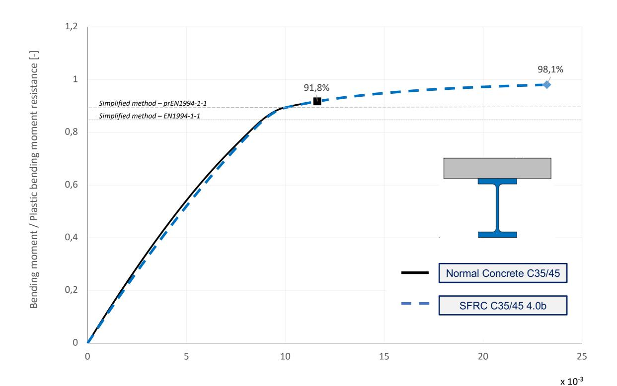
Curvature of the cross-section [1/m]
