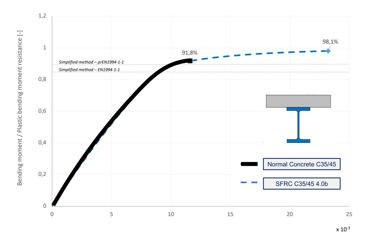
Curvature of the cross-section [1/m]
